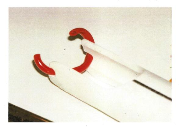
Cut a piece of 1" PVC pipe to desired length. Remember that to increase the overall length of the finished spiral applicator, it can be slipped over a broom or mop handle. Or cuppled with another piece of PVC pipe.
